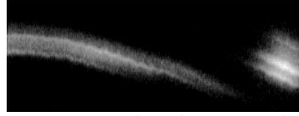
figure 10 : cw laser becoming pulsed, horizontal time scale : 10 ms, vertical time scale : 700 ps,  $I = 35 \text{ mA}$ .
