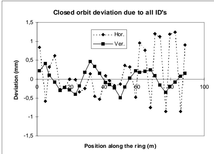
Figure 1. Closed orbit deviation with all ID's closed.
