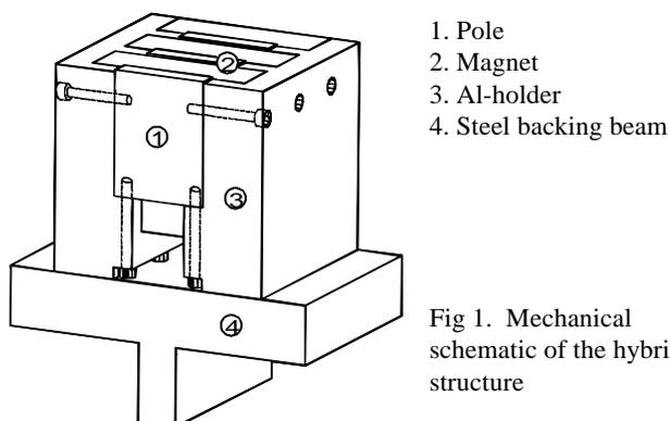
Fig 1. Mechanical schematic of the hybrid structure
