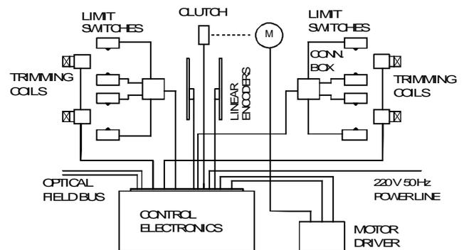
Fig 2. Schematic of the undulator control system
