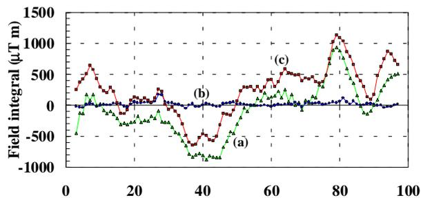
Fig 3. The field integrals of U5.2 derived by: (a) Hall probe measurement, (b) calculation with homogeneously magnetized blocks and (c) calculation with 16-sub-block model
