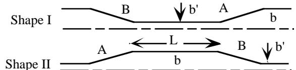
Figure 3. The shape for simulation. Shape I is actual convex shape at ID sections or absorbers. Shape II is for the simulation
