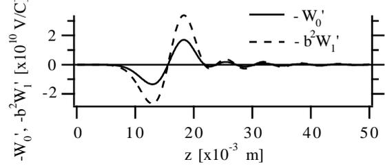
Figure 2. The wake functions for a fringe. The bunch length is 3mm(r.m.s.). The shape of two wake functions,  $V_0^{\parallel} = -W_0'$  and  $V_1^{\parallel} = -b^2 W_1'$ , are the same and scale is factor 2. From Eq. (4), this result shows Eq. (2) is valid for the impedance of fringe and  $d=b$ .
