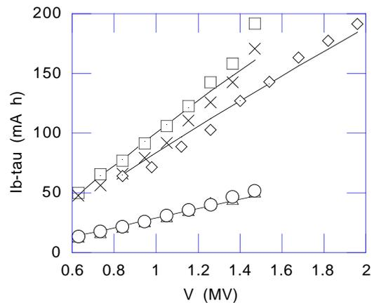
Figure 1. Product of beam current (mA) and lifetime (hours) at 2 GeV as a function of r.f. voltage for three different currents (10, 7, 6 mA) and coupling (2%, 0.85%, 0.16%). The solid lines correspond to the prediction.
