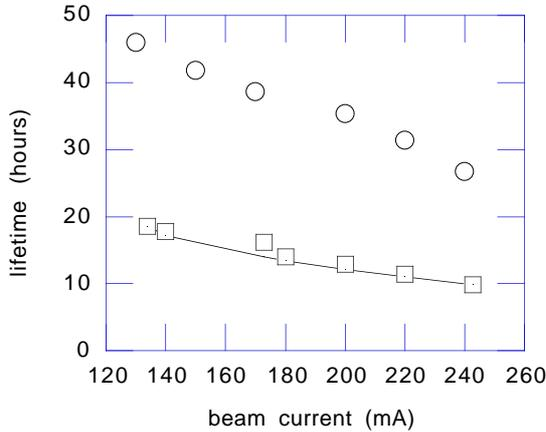
Figure 2. Lifetime as a function of beam current for the high lifetime mode (circles) and low lifetime i.e. instability free mode (squares) for 80% (i.e. 346 bucket) filling at 1.76 MV. Solid line is the prediction.
