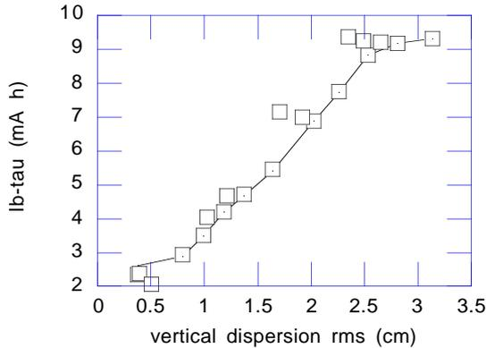
Figure 6. Product of beam current (mA) and lifetime (hours) at 2 GeV as a function of rms vertical dispersion for a single bunch currents between 3 and 6 mA. The solid line is the coupling fitted prediction.
