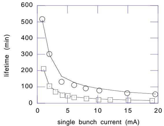
Figure 5. Beam lifetime at 2 GeV as a function of single bunch current for two different r.f. voltages (circles 1.76 MV and squares 0.84 MV). Solid line is the prediction.
