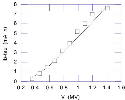
Figure 3. Product of beam current (mA) and lifetime (hours) at 2 GeV as a function of r.f. voltage for a single bunch current of about 2 mA. Solid line is the prediction.
