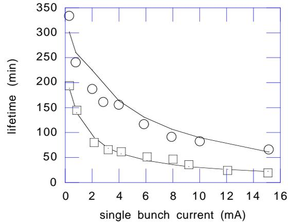
Figure 4. Beam lifetime at 1 GeV as a function of single bunch current for two different r.f. voltages (circles 1.76 MV and squares 0.84 MV). Solid line is the prediction.
