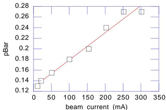
Figure 8. Ring pressure as a function of beam current at 1 GeV. The solid line is the linear fit to obtain the desorption  $P_1$ .
