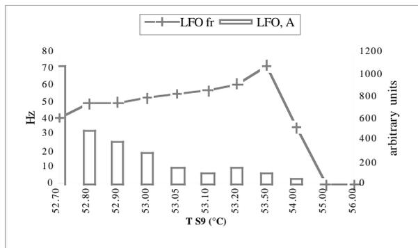
Figure 5: Growth rate of Coupled Bunch Mode 363 (for 150 mA at 2 GeV) as a function of cavity temperature (a) and the corresponding change in frequency and amplitude of the relaxation oscillation (b). In figure (b) also the lifetime is reported.
