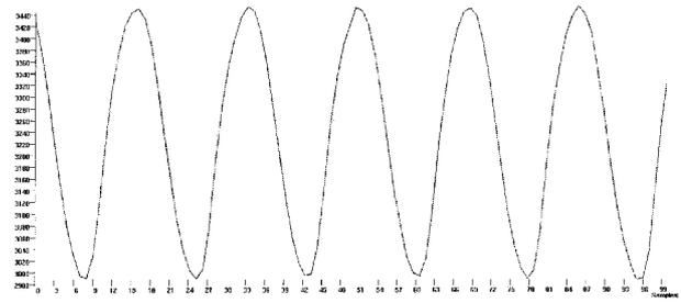
Figure 4: BPM button signal for medium CBI excitation.
