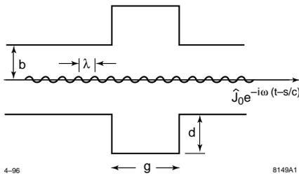
Figure 1: Schematic view of a short cavity
