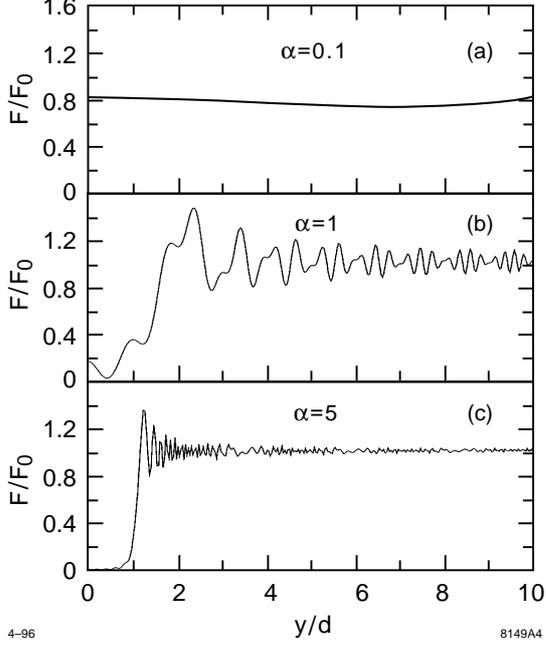
Figure 4: Energy flux  $F/F_0$  as a function of transverse position at various distances  $z \propto 1/\alpha^2$  behind the step-out.
