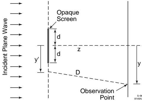
Figure 3: Diffraction of plane wave on a screen.
