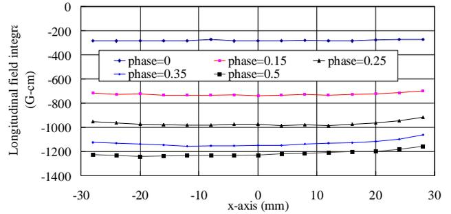
Figure: 6 Longitudinal field integrated strength as a function of x at different phase. The dipole strength has been changed but the higher multipole strength is fixed when the phase is changed.
