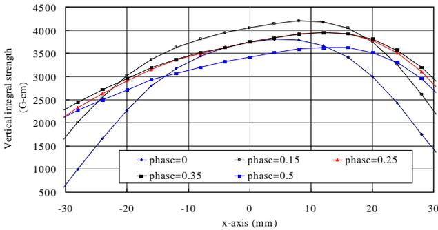
Figure: 5 Vertical field integrated strength as a function of x at different phase (without any shim or magic finger correction). The dipole and the higher multipole strength have been changed when the phase is changed.
