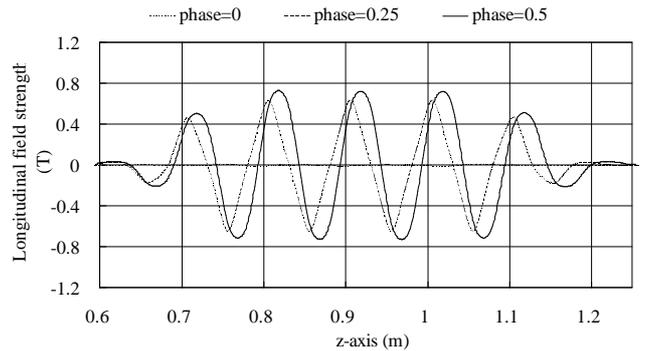
Figure:2 The on-axis  $B_z$  magnetic field was measured at gap  $g=22$  mm and change the phase. The  $B_z$  field is maximum at phase  $\theta = 0.5$ , and is zero at phase  $\theta = 0$ .
