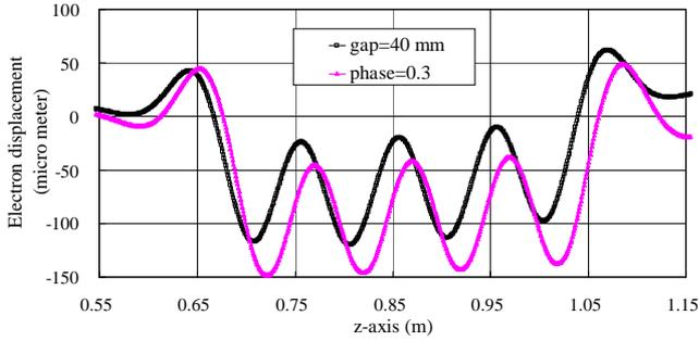
Figure: 3 The electron trajectories are calculated at the same  $K=5.07$  value but under the different phase and gap. One is at gap=22 mm and phase  $\theta = 0.3$ , and the other one is at gap=40 mm and phase  $\theta = 0$ .
