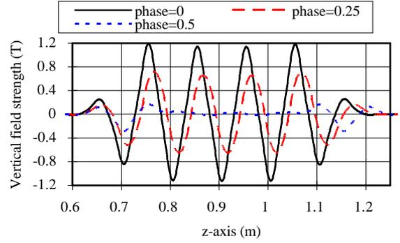
Figure:1 The on-axis  $B_y$  magnetic field was measured at gap  $g=22$  mm and change the phase. The  $B_y$  field is maximum at phase  $\theta = 0$ , and is zero at phase  $\theta = 0.5$ .
