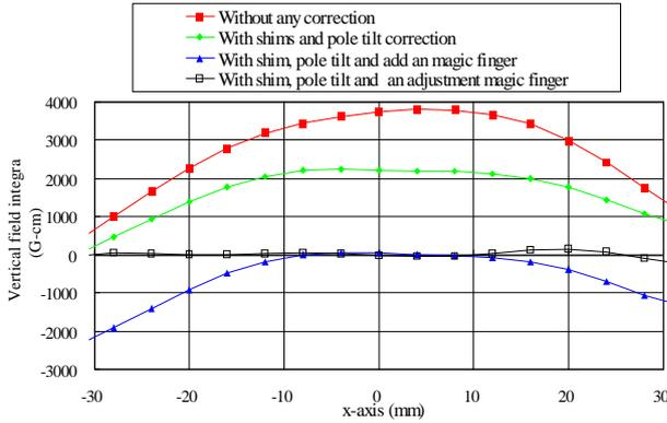
Figure: 4 The integral field strength as a function of x for the different kind of correction skill at gap= 22 mm and phase=0.
