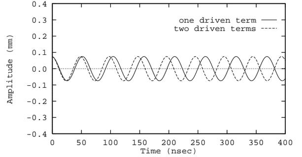
Figure 1: Comparison of  $H_2^+$  ion vertical oscillation at one  $\sigma_y$  amplitude as one driven force term and two driven terms considered
