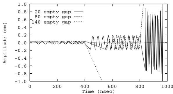
Figure 2: Motion of  $H_2^+$  ion under the force of different number of electron bunches
