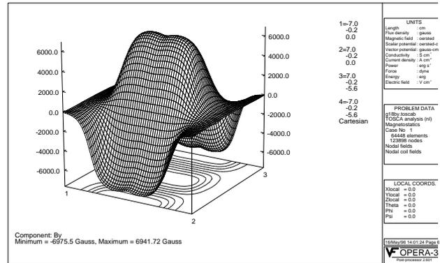
Figure 3: Profile of the vertical magnetic field in the middle plane (x-z plane with y=0).
