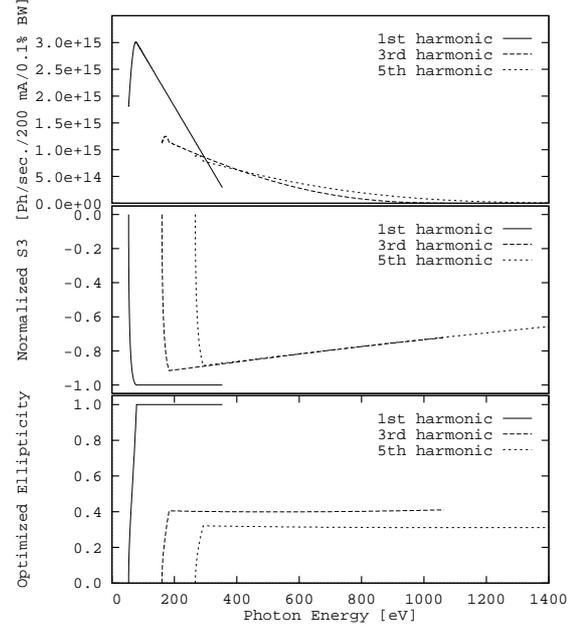
Figure 4: Elliptically polarized undulator spectrum, under condition of the maximal achievable merit function, for the SRRC device EPU5.6.
