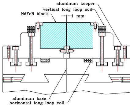
Figure 2: Side view of the SRRC device EPU5.6 with long-loop correction coils.
