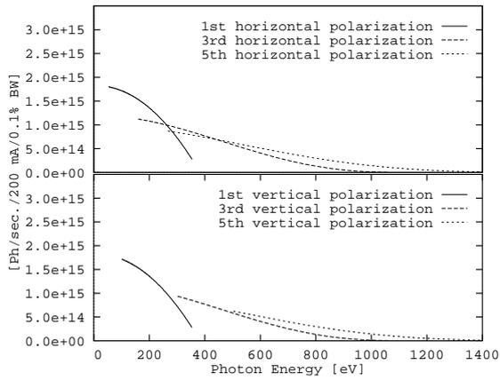
Figure 1: Linear polarized undulator spectrum for the SRRC device EPU5.6.
