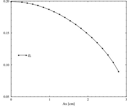
Figure: 4 Tune versus amplitude in the horizontal plane.
