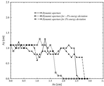
Figure: 7 Machine dynamic aperture with W95 in.
