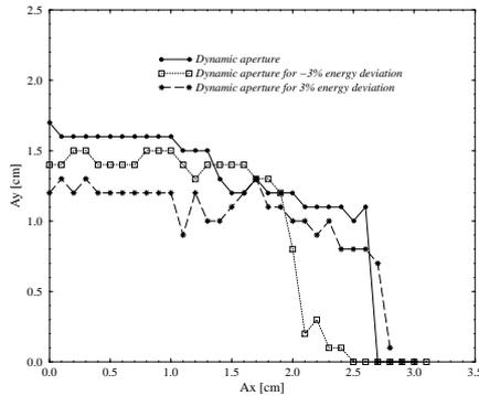
Figure: 6 Machine dynamic aperture with U60 in.
