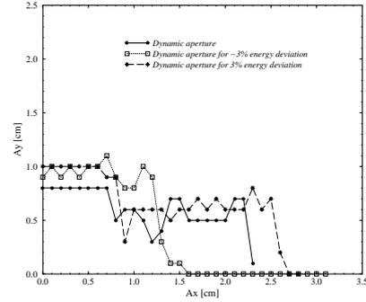
Figure: 8 Machine dynamic aperture with W180 in.
