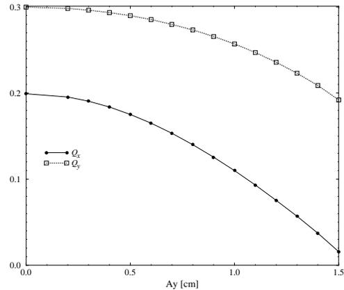
Figure: 5 Horizontal and vertical tune versus vertical amplitude.
