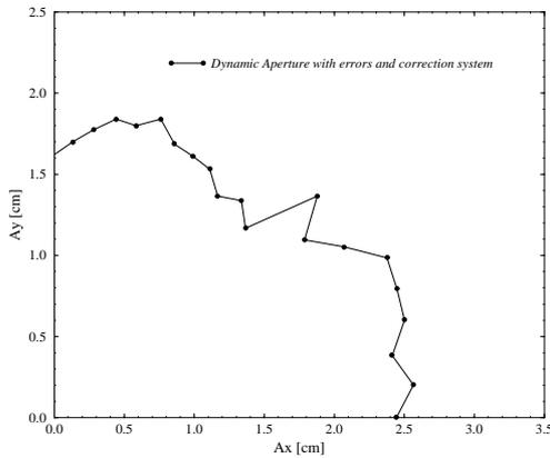
Figure: 2 Dynamic aperture with orbit errors and correction system.
