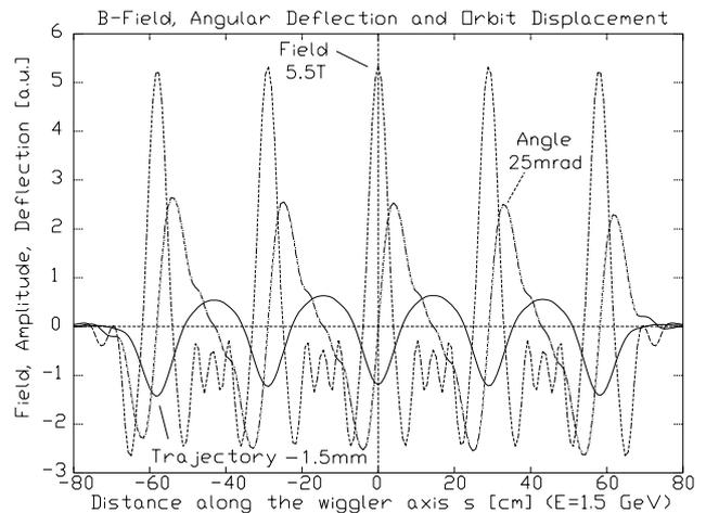
Figure 1: Magnetic field, angular deflection and orbit displacement along the wiggler axis (asymmetric mode)
