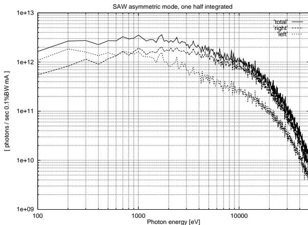
Figure 3: Spectrum of the asymmetric mode
