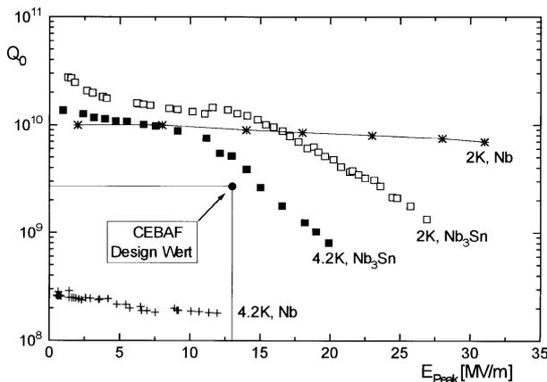
Fig. 4: Field dependence of the quality factor of one of the single-cell 1.5 GHz cavities as measured before (Nb) and after Nb<sub>3</sub>Sn coating at 2 and 4.2 K. The CEBAF design value is marked for comparison.
