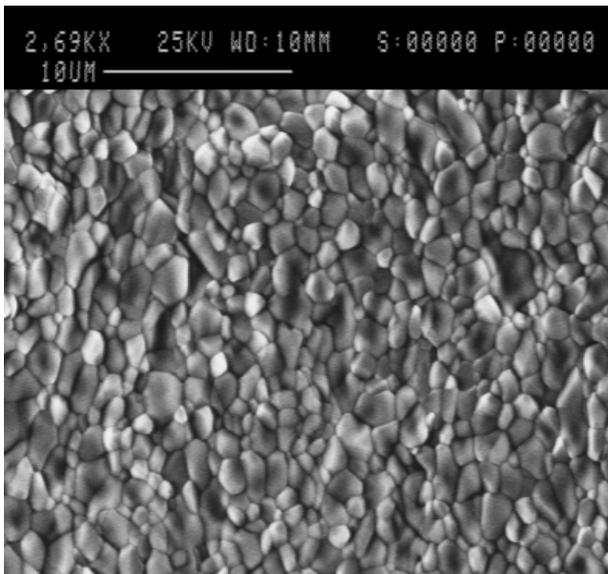
Fig. 2: SEM picture of a typical  $Nb_3Sn$  surface as grown for 3h on a high purity Nb sample.
