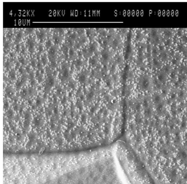
Fig. 1: SEM picture of a high purity Nb sample with Sn nuclei, which were formed by means of SnCl<sub>2</sub> at 200°C.
