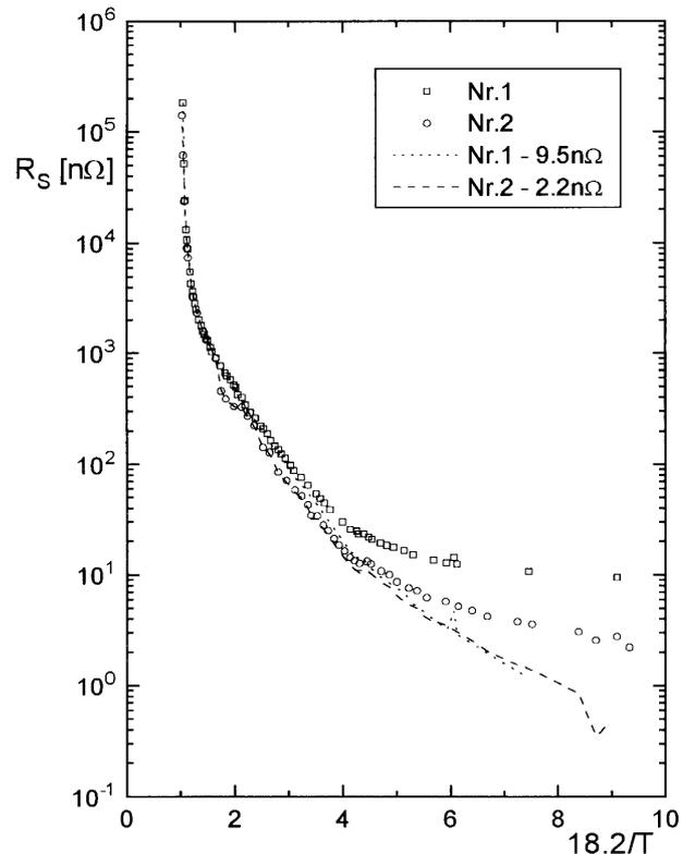
Fig. 3: Temperature dependence of the surface resistance of two  $Nb_3Sn$  coated single-cell 1.5 GHz cavities. The lines result for subtraction of the residual  $R_s$  values at 2 K.
