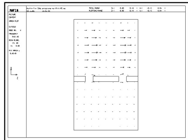
Figure 6: E-field Simulation of  $\pi$ -Mode Structure
