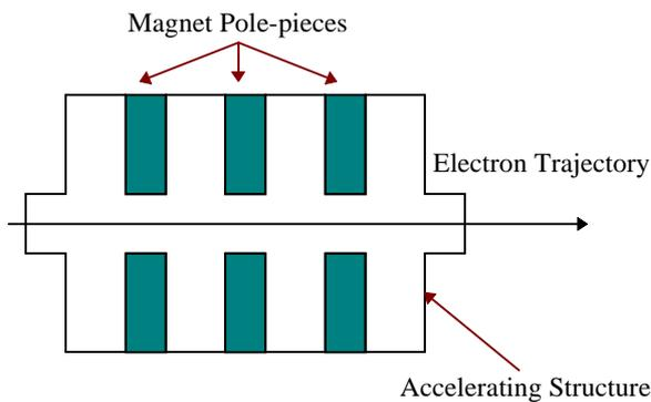
Figure 1: Muffin-tin Accelerating Structure
