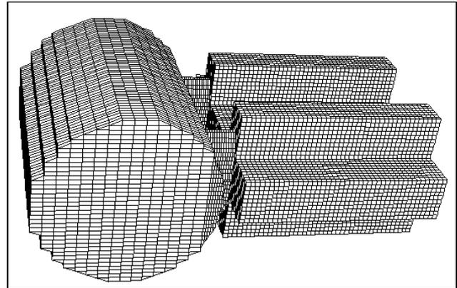
Figure 5: Side-coupled  $\pi$ -Mode Structure
