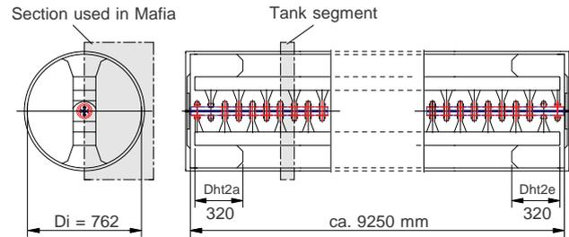
**Fig.1:** Schematic cross sections of the RFQ accelerator
