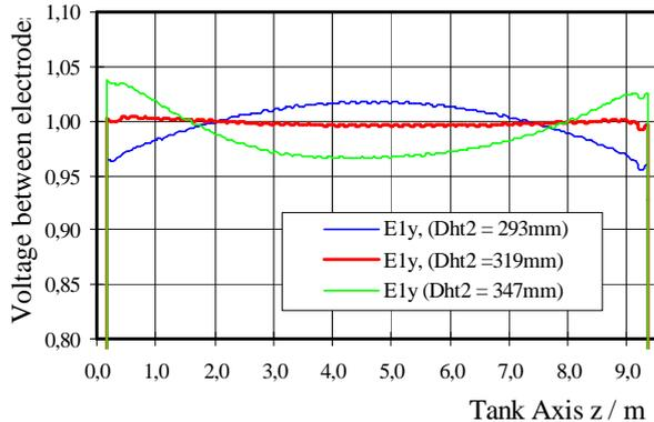
**Fig.5:** Voltage distribution vs. z-axis ( $x=2\text{mm}$ ,  $y=4\text{mm}$ ) Flat curve for optimum end window length  $Dht2=319\text{mm}$
