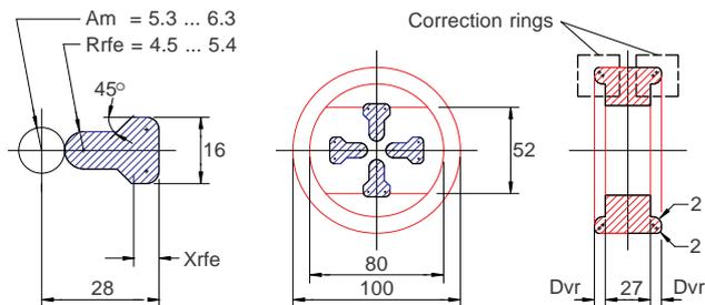
**Fig.2:** RFQ electrodes with carrier rings and correction elements for compensation of the capacity variations
