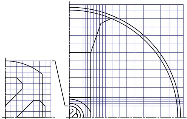
**Fig.4:** Mafia mesh m4, mesh densities from 4.0...30 mm Simplified RFQ electrode geometry and mesh used for calculations including the complete tank length. Mesh lines around the electrodes shown only in the left part.
