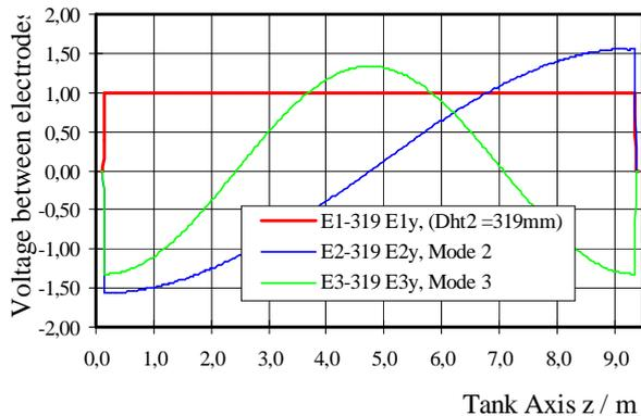
**Fig.6:** Voltage distributions vs. z-axis ( $x=2\text{mm}$ ,  $y=4\text{mm}$ ) Calculations for the lowest resonant modes F1, F2, F3.
