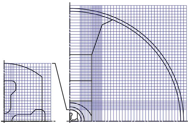
**Fig.3:** Mafia mesh m1, mesh densities from 1.0..10 mm RFQ electrode geometry used for investigation of short elementary tank slices. Mesh around the RFQ electrodes is shown only in the 5x enlarged part on the left side
