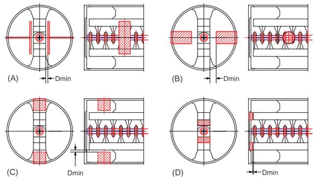
**Fig.7:** Tuning ranges of different tuning elements
