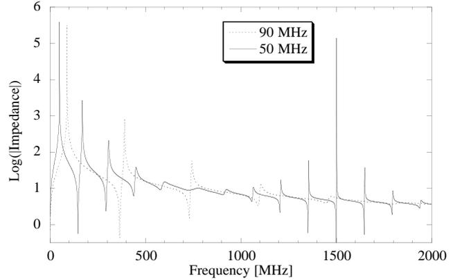
Figure 4: Longitudinal impedance[ $\Omega$ ] of the cavity which is tuned at 50 MHz or 90 MHz.
