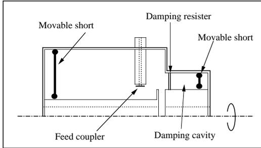
Figure 2: Functional structure of the coaxial cavity.
