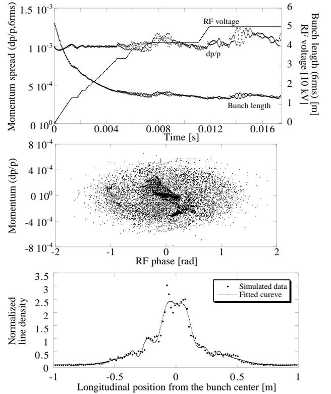
Figure 1: Beam bunching of a 150 MeV/u  $\text{U}_{238}^{92+}$  beam of  $4.5 \cdot 10^6$  ions per bunch. The longitudinal phase space plot and the line density are at the end of the simulation.
