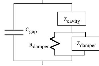
Figure 3: Approximate longitudinal equivalent circuit of the cavity.
