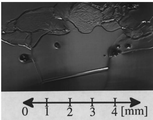
Figure: 3 A photograph of the welding imperfections, porosities on the equator EBW seam, found at the heating region in the M-1 cavity .
