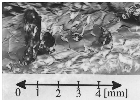
Figure: 7 A photograph of the sputtering balls on the iris EBW seam found at the heating region in the M-5 cavity.
