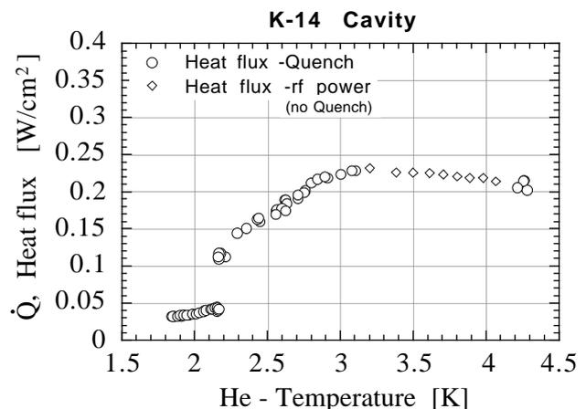
Figure: 5 Temperature dependence of the heat flux at the quench fields.
