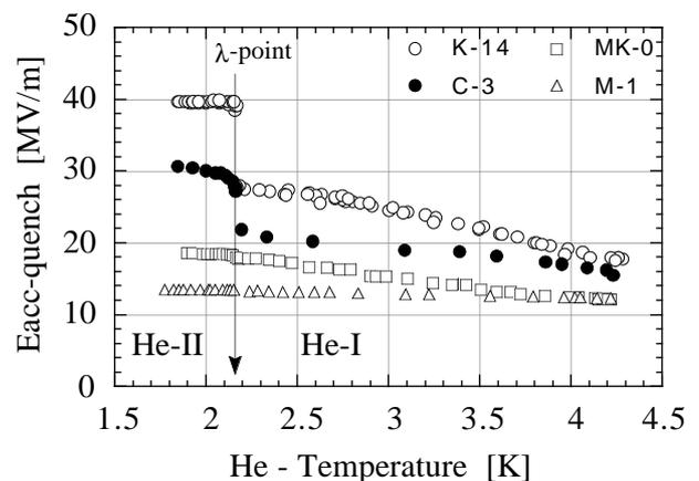
Figure: 1 Temperature dependence of the quench field between 1.8 K and 4.2 K in four cavities.
