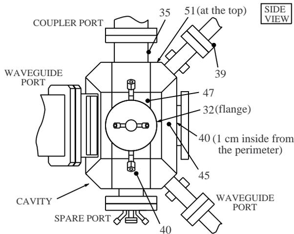
Fig. 3. Measured temperatures ( $^{\circ}\text{C}$ ) of the cavity under an input power of 50 kW. Input water temperature,  $31^{\circ}\text{C}$ .
