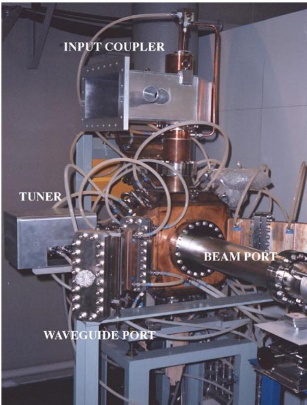
Fig. 1. High-power test cavity mounted on a test bench.
