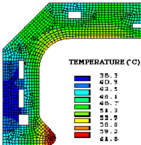
Fig. 4. Result of a thermal analysis on the axisymmetrical cavity model using the ANSYS code. Assumed a dissipated power of 50 kW/cavity, water temperature of  $30^{\circ}\text{C}$  and a heat-transfer coefficient of  $1.2 \text{ W/cm}^2/\text{K}$  on the cooling channels.
