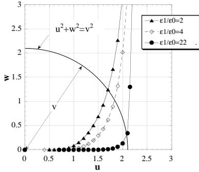
Figure 6: The values of  $u$  and  $w$  of the  $HE_{11}$  mode ( $n=1$ ) are obtained by numerical calculations. A quarter of the circle is given by equation (4-2).
