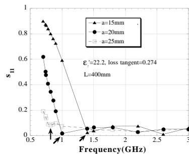
Figure 2:  $S_{11}$  frequency response curves for the HOM absorbers with  $a=15, 20,$  and  $25$  mm. Closed circle for the SiC absorber ( $a=20$  mm) employed in the accelerating cavity.
