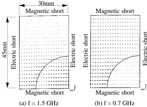
Figure 5: Electric field of the propagating mode in the 2-dimensional lossless model. ( $a=20\text{mm}$ ,  $\epsilon_r=22$ ).
