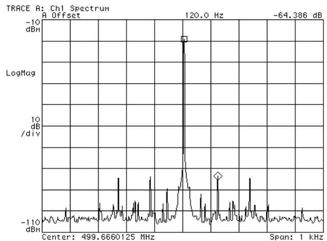
Figure 2. Spectrum of rf signal picked up from cavity
