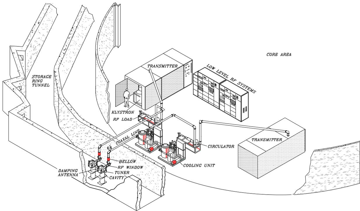
Figure 1. Layout of the SRRC/TLS RF System
