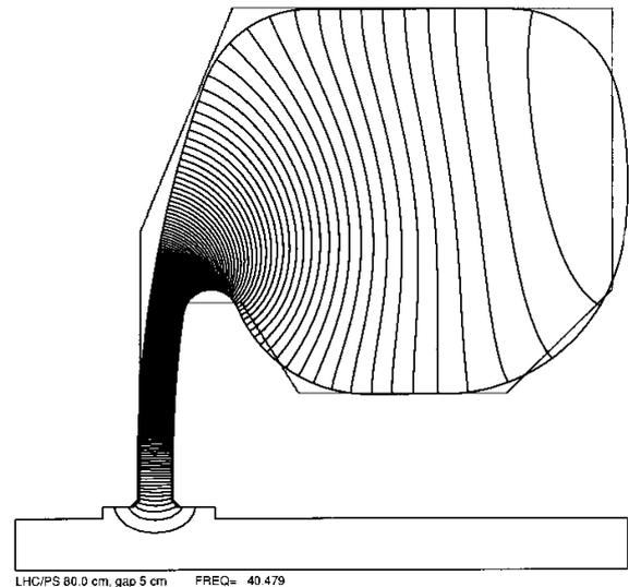
Figure 1 : SUPERFISH plot of 40 MHz cavity mode for the CERN cavity. Outline of the wooden model is also shown.
