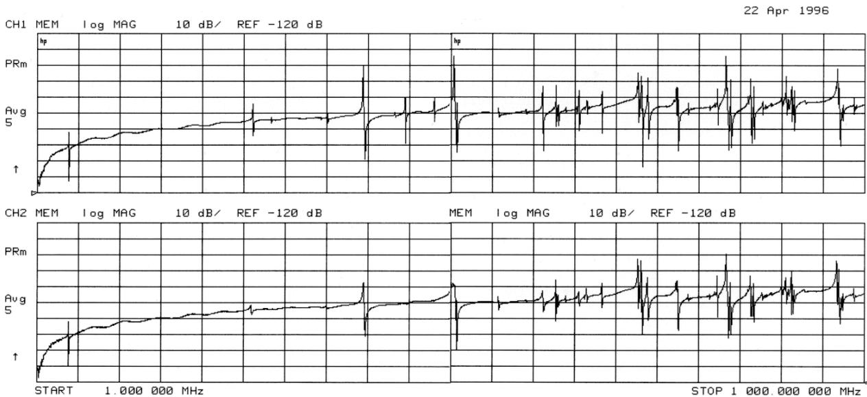
Figure 3 : Frequency spectrum of the model cavity with and without HOM dampers.
