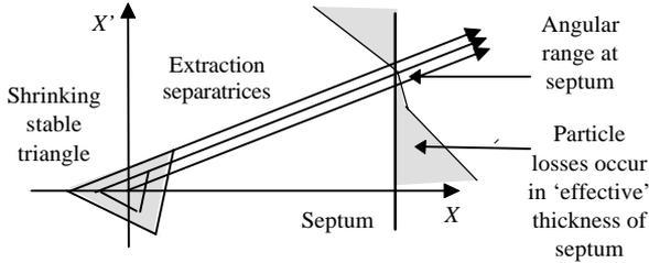
Figure 3: Movement of the extraction separatrix.
