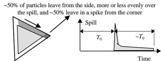
Figure 5: An elementary ‘strip’ spill.
