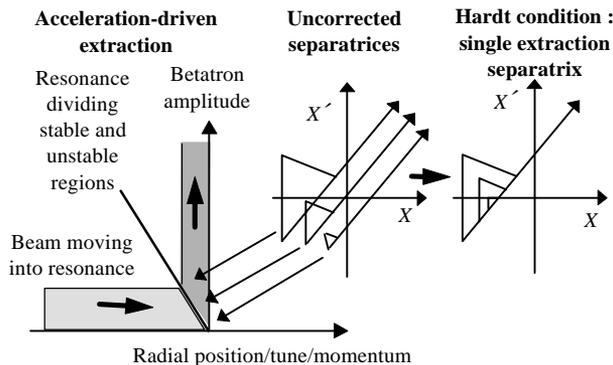
Figure 4: The Hardt condition.
