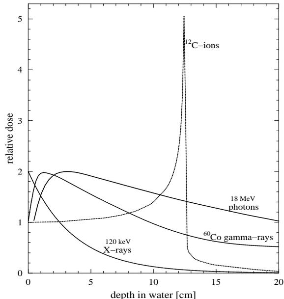
Fig.1 Comparison of depth dose profiles of X-rays, Co-gamma-rays and electron Bremsstrahlung with a carbon beam showing an inversed dose profile with the maximum energy deposition at the end of the range.
