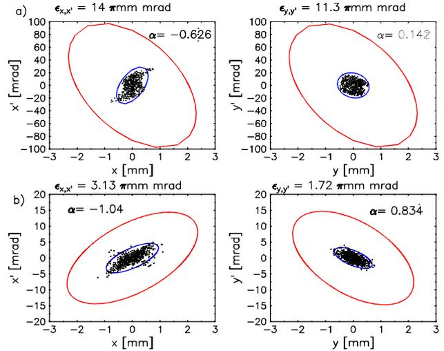
Figure 2: Emittances at the entrance and at the exit of the REX-ISOLDE-RFQ concerning a real beam from the mass separator. The emittances given in Table 1 are the larger ellipses. The emittance values in the graphic are represented by the small beam ellipses.
