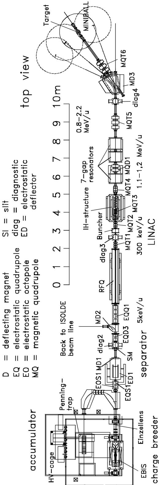
Figure 1: Layout of the REX-LINAC.
