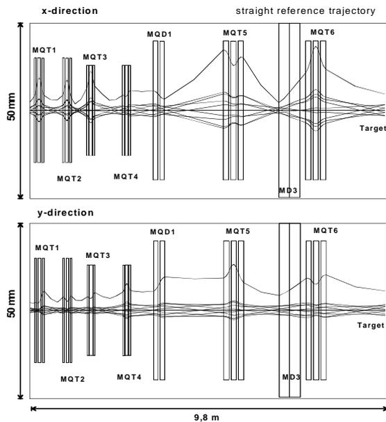
diverging with a maximum slope of about 2 mrad. Figure 4: Calculation of the beam transport of a 300 keV/u beam out of the RFQ to the target of REX-ISOLDE concerning the exit emittances from the RFQ.
