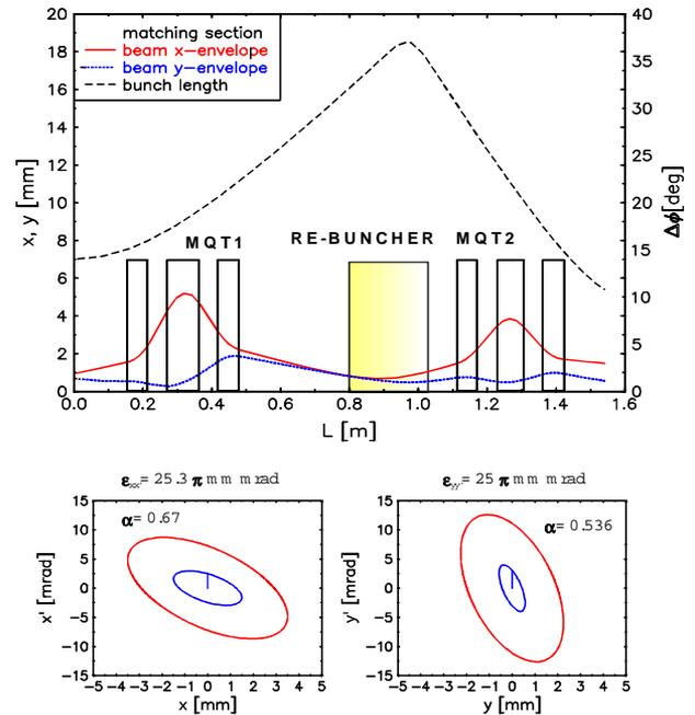
Figure 3: Calculation of the matching section between the RFQ and the IH-structure. The transverse emittances of the real beam are in comparison to the design emittances at the entrance of the IH-structure.
