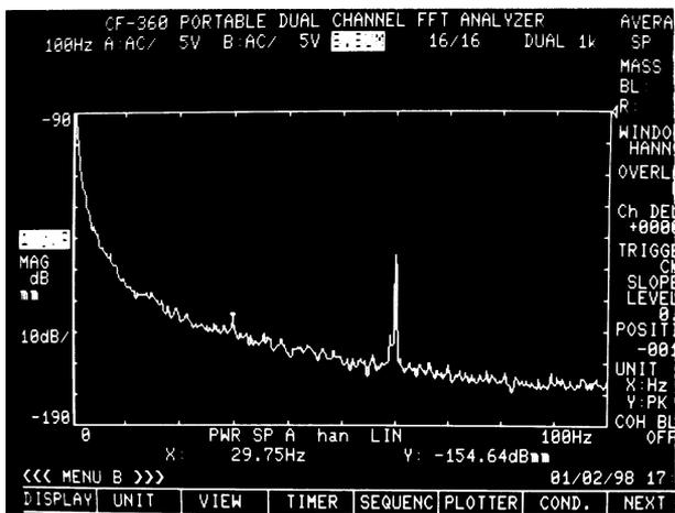
Figure 5: The upper photo is a spectrum of vibration with the cyclic phase shift motion on the floor near the ID23. The lower one is in all motor-off of the ID23. The peak at 41.25 Hz is caused by the phase motion in the upper photo. Its amplitude is 0.62 nm.
