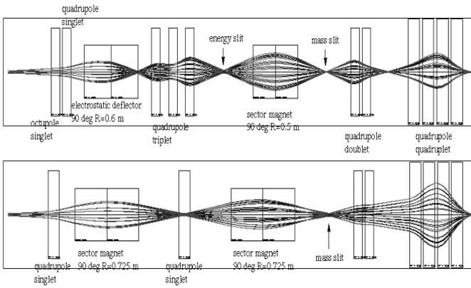
Figure 1: Straight optical axis representation of the achromatic system (upper figure) and the magnetic system (lower figure) calculated with COSY INFINITY. The calculated trajectories are shown only in the dispersive plane. All quadrupoles are electrostatic. The optical axis has a length of 8528 mm for the achromatic system and 8746 mm for the magnetic system, measured from the EBIS delivering point (left) to the RFQ entrance point (right).
