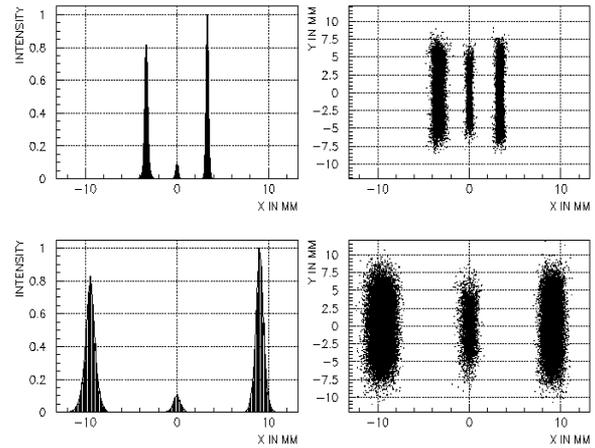
Figure 2: The ion beam at the mass slit is calculated with the MONTECARLO method. Here 100000 particles are transformed through the COSY INFINITY third order transport matrix. The upper picture shows the conditions at the mass slit of the achromatic system. Analogous the lower picture for the magnetic system. The particles have the mass deviations  $-1/150$ ,  $0$  and  $+1/150$ . The relative number of particles for the three masses are  $10:1:10$ .
