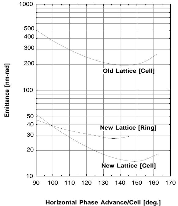
**Figure 2:** Emittance curve for old and new lattice. The natural emittance is shown as a function of horizontal phase advance of the normal cell. Upper curve is for old lattice. The lower two are for new one. Lines indicated as 'Cell' are curves for normal cells only. 'Ring' is for the whole ring (including the contribution from other parts).
