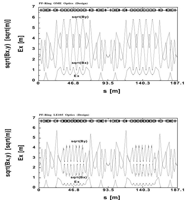
**Figure 1:** Old (upper) and new (lower) optics(105 degree). There are large changes in the normal cell sections but very little in remainder parts.
