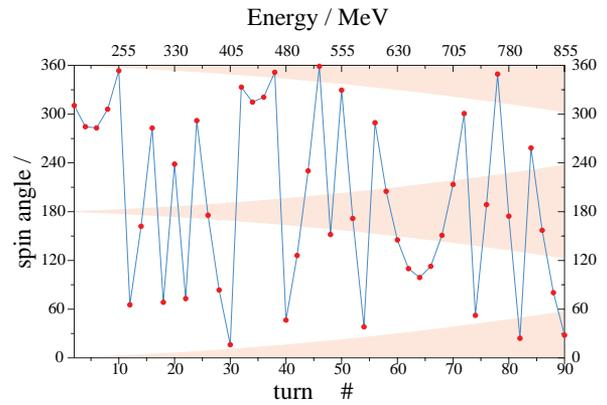
Figure 2: Spindirection in experimental hall A1 for extraction; case of standard accelerator adjustment. The grey regions symbolize the areas, where a longitudinal spindirection may be adjusted by slight ( $\leq 0.15$  %) energy variation.
