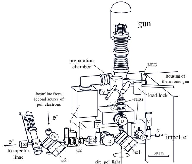
Figure 1: MAMI - source of polarized electrons at the injection point.  $\alpha$ : alphas magnet, D: diff. pumping stage, E: emittance filter, I: ion getter pump, Q: quadrupol, S: solenoid, V: all metal valve, W: wire scanner
