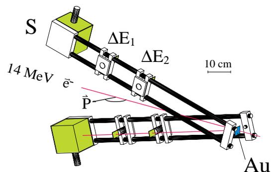
Figure 3: The 14 MeV Mott - polarimeter
