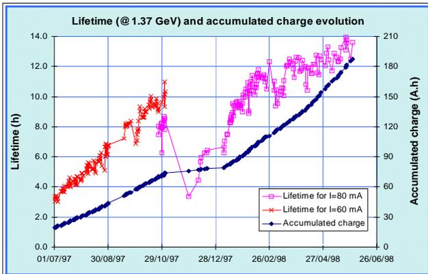
Figure 2: Evolution of beam lifetime and accumulated charge in the LNLS first year of operation.
