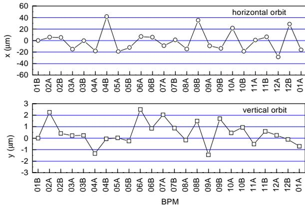
Figure 3: Reproducibility of the horizontal (top) and vertical (bottom) orbits after correction to a reference orbit.
