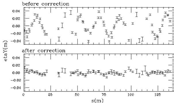
Fig. 4, Measured vertical dispersion in the ring before dispersion correction (top) and after correction (bottom).
