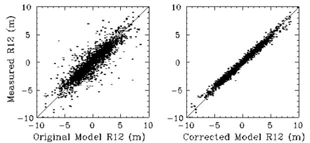
Fig. 1, Measured  $R_{12}$  vs. calculated  $R_{12}$  using the original model (left) and the corrected model (right).
