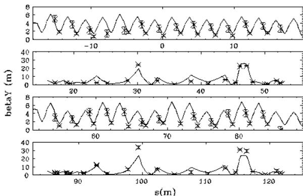
Fig. 2, Measured (plots) and model (lines) vertical beta function.
