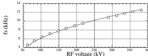
Fig. 5, Measured synchrotron frequency vs. RF voltage (plot), the line shows calculation from the model using fitted momentum compaction factor.
