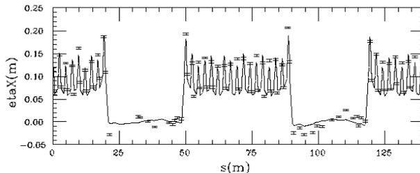
Fig. 3, Measured horizontal dispersion in the ring (plot) and model calculation (line).
