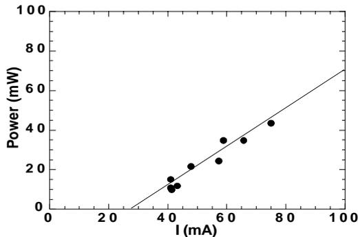
figure 8 : total laser power (black points), transmitted through both sides of the optical cavity, versus the total current stored in the ring and a linear fit (plain line).
