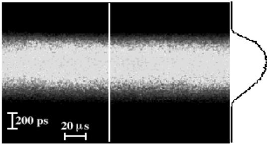
figure 3 : Double sweep streak camera image, horizontal range = 200  $\mu$ s, vertical range = 1.7 ns,  $I = 80$  mA with the quadrupolar feedback damping the quadrupolar coherent synchrotron oscillation, the bunch shape does not oscillate anymore as in figure 1.
