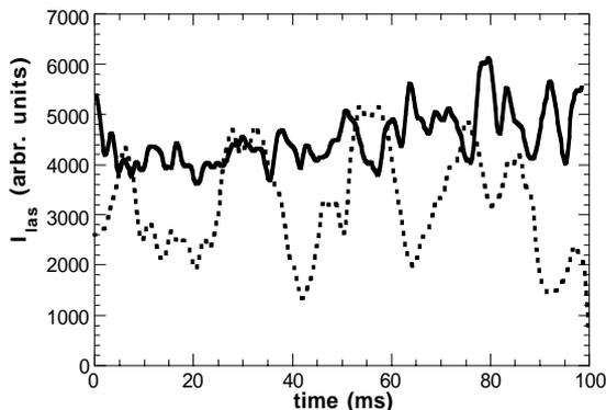
figure 9 : laser intensity ( $I_{las}$ ) versus time. Without feedback (dashed line), the laser macrostructure is unstable
