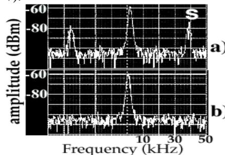
figure 7 : measurements of the sidebands with a spectrum analyser. In a), FEL is off, presence of sextupolar coherent synchrotron oscillations (S) at 36.8 kHz. In b), FEL on, the sextupolar modes are damped.
