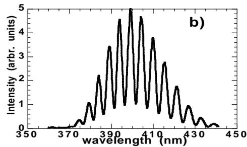
figure 5 : FEL optical klystron spectra at high current. In a), the spectrum is degraded by quadrupolar oscillations, in b) with the quadrupolar feedback, the spectrum is normal.
