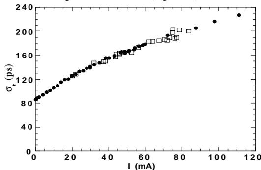
figure 4 :  $\sigma_e$ , RMS bunch length versus the total current in the ring, (●) quadrupolar feedback off, (□) quadrupolar feedback on.
