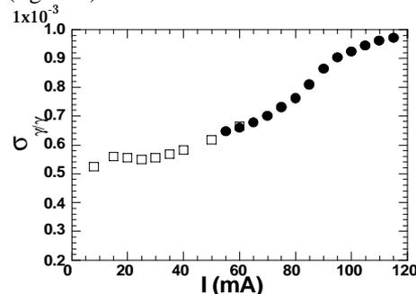
figure 6 : energy spread  $\sigma_{\gamma/\gamma}$  versus the total current  $I$ , quadrupolar feedback off (□) and quadrupolar feedback on (●) measured using the optical klystron fringe method.
