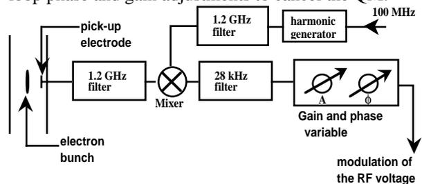
figure 2 : Scheme of the feedback damping the quadrupolar coherent synchrotron oscillations.
