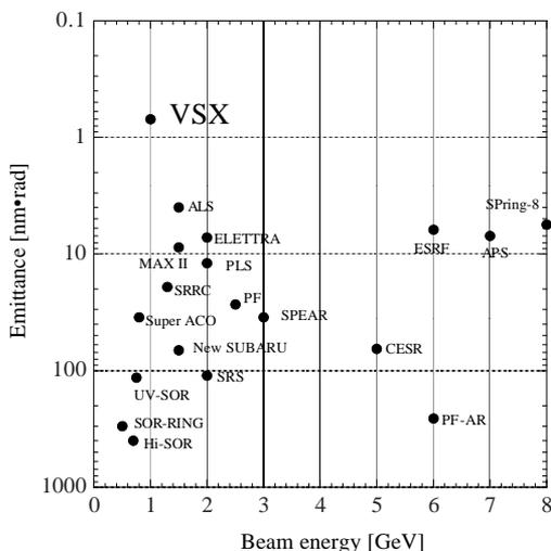
Figure 1: The emittance of synchrotron radiation light sources.
