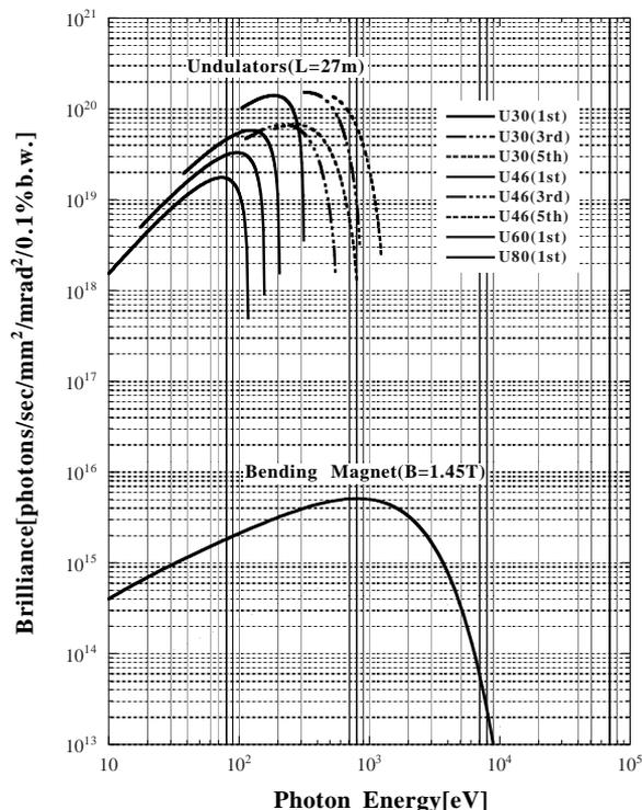
Figure 2: The brilliance of VSX Energy = 1.0 GeV, Current = 200 mA, Emittance = 1.52 nm•rad and Coupling = 10% are assumed. The emittance growth due to intrabeam scattering is taken into account.
