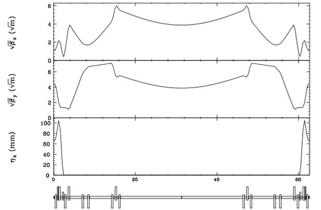
Figure 6: The optics of the *M-M'* Section.
