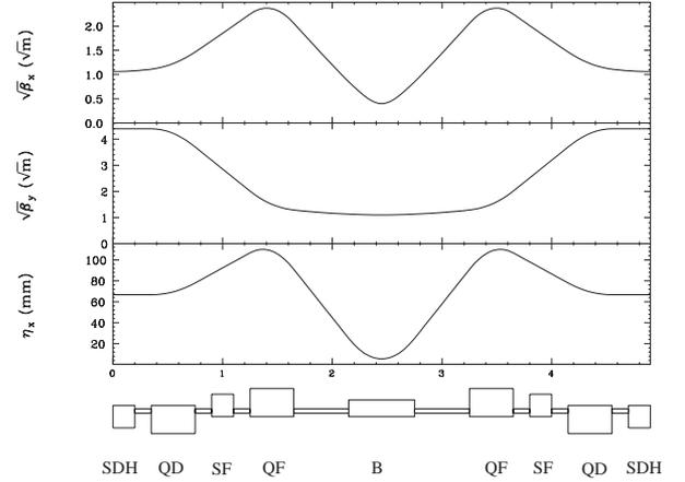
Figure 5: The optics of the *Normal* cell.
