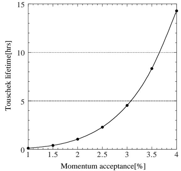
Figure 8: The momentum acceptance vs. Touschek lifetime. Energy = 1.0 GeV, Beam Current = 200 mA, RF bucket height = 4% and Coupling 10% are assumed.
