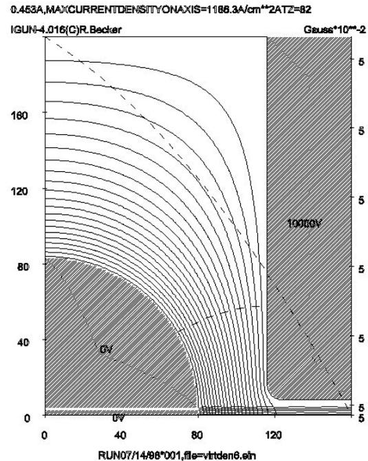
Fig. 5. Simulation of the electron gun for  $1000 \text{ A/cm}^2$  as a whole, showing the field line (lower dashed line) to cut out the cathode part for a simulation with finer mesh in Fig. 6
