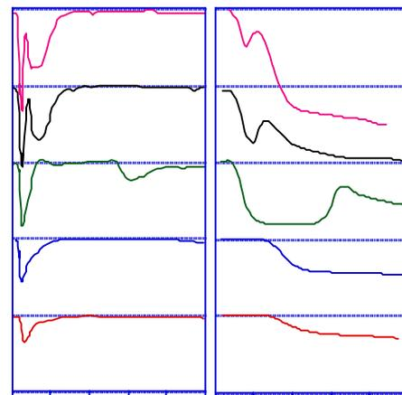
Fig. 3. The sequences of the electron accumulation pulse (left) and the anode current (right). The heat power to the electron gun emitter is increasing upwards in the diagram.
