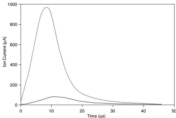
Fig.1. Ar ion current pulse as measured from RefEBIS Faraday cup before the phase transition (lower trace) and after the phase transition (upper trace) to the string state.
