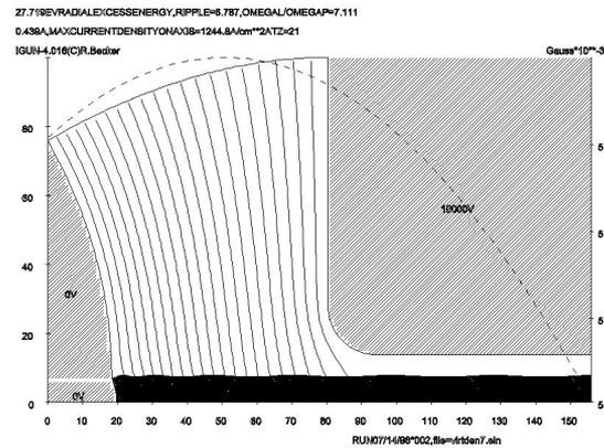
Fig. 6. Simulation of the electron gun of Fig. 5 with higher mesh resolution in the vicinity of the Z-axis.
