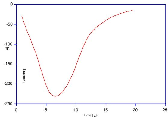
Fig. 2. The induced electron current pulse from the drift tube structure during the phase transition.
