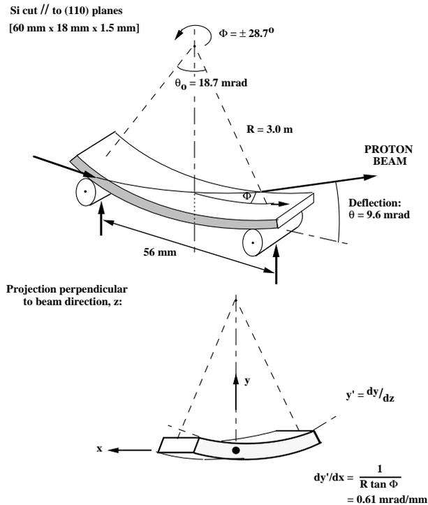
Figure 3: Schematic arrangement of the bent crystal
