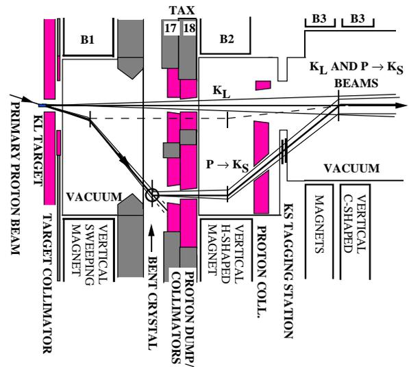
Figure 2: Schematic layout of the  $K_L$  target station
