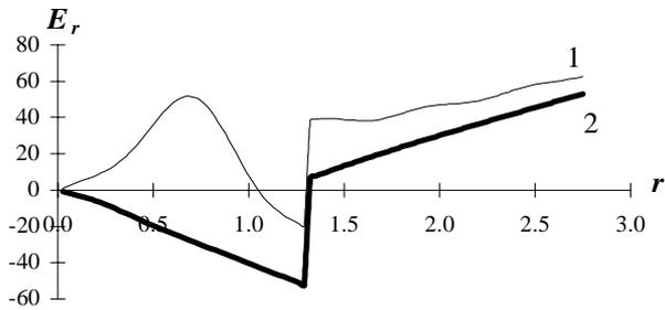
Fig. 2. Dependence of the net radial electric field on radius for an ion current of 4 A (curve 1) and 30 mA (curve 2).
