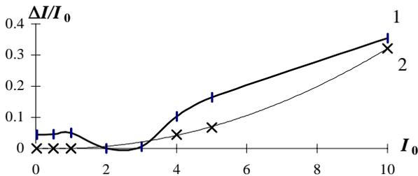
Fig. 3. The plot of relative losses of ion beam current versus input current (1 -  $E_z=56$  kV/cm; 2 -  $E_z=27$  kV/cm)
