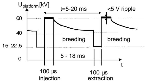
Figure 3. REXEBIS platform potential relative ground during two cycles.
