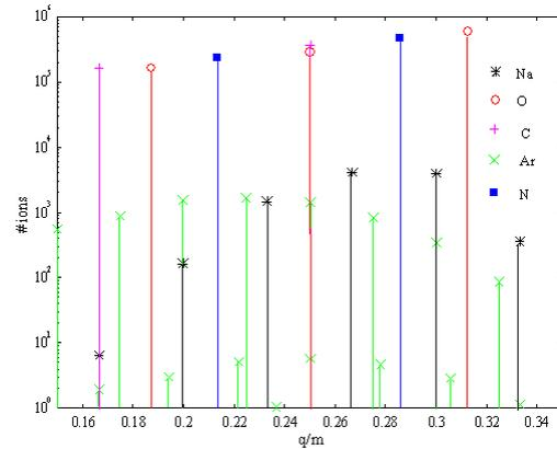
Figure 4. Calculated  $q/A$  spectrum showing the absolute number of extracted residual and radioactive ions per pulse. Breeding time 13 ms; 10 000 injected <sup>30</sup>Na ions.
