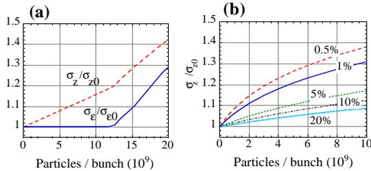
Figure 5: Estimation of bunch lengthening at energy 1.3 GeV. (a) by potential well distortion, (b) by intra-beam scattering.
