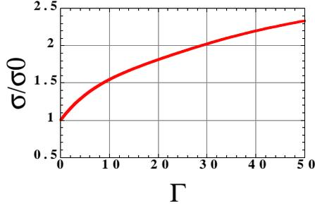
Figure 2: An inductive impedance: the bunch length variation as a function of  $\Gamma$ .
