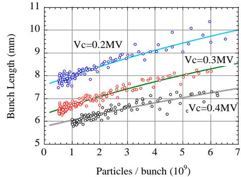
Figure 4: Measured bunch length as a function of the bunch intensity. Curves show the fitting results
