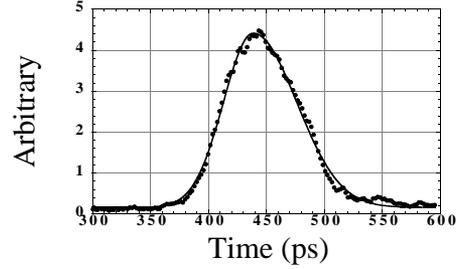
Figure 3: Longitudinal bunch shape at  $V_c=300\text{kV}$  and bunch intensity of  $5 \times 10^9$  ppb.
