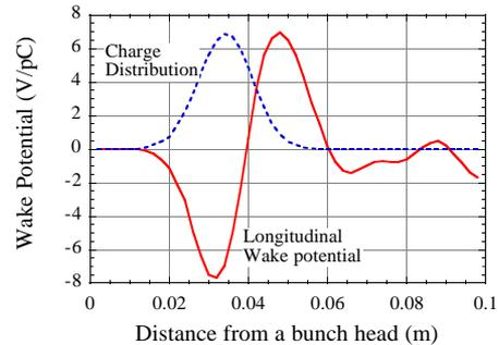
Figure 1: Total longitudinal wake potential in ATF damping ring.
