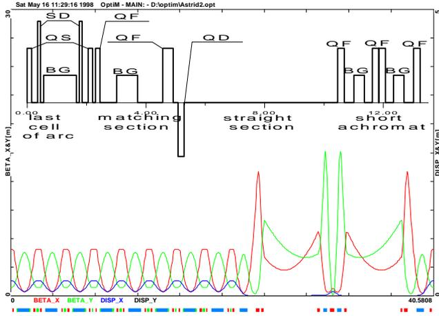
Figure 1. The lattice of arc, matching section and straight section (QF, QD –focusing and defocusing quadrupole, QS-focusing quadrupole incorporated with sextupole, SD-defocusing sextupole, BG-combined function bend magnet with negative gradient).
