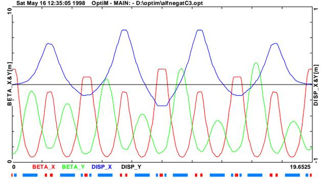
Figure 3. The arc lattice with tunable momentum compaction factor.
