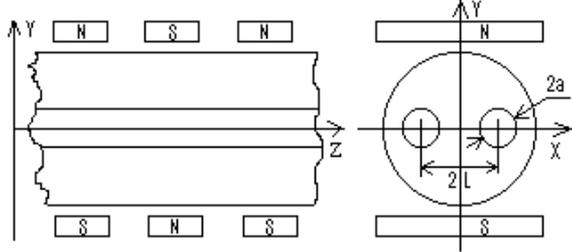
Figure 1: Cross-section of RF system and M- undulator. For plane magnetic undulator
