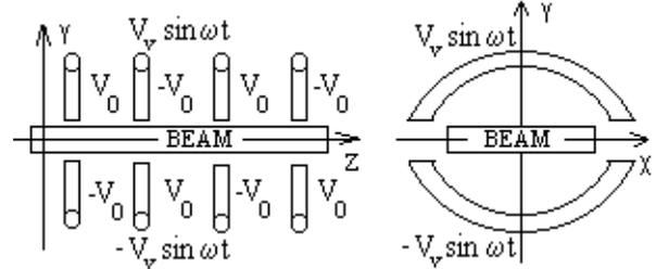
Figure 2: Cross section of RF-system and E- undulator.
