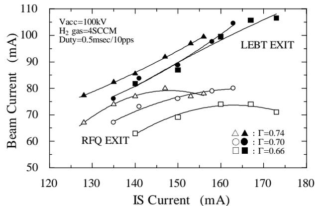
Figure 2 : Peak beam current at the LEBT exit and the RFQ exit as a function of the IS current.
