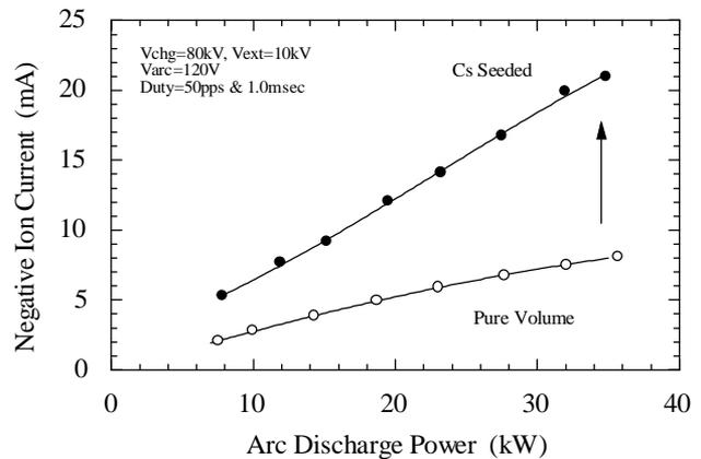
Figure 5 : Negative ion current as a function of the arc discharge power with and without cesium.
