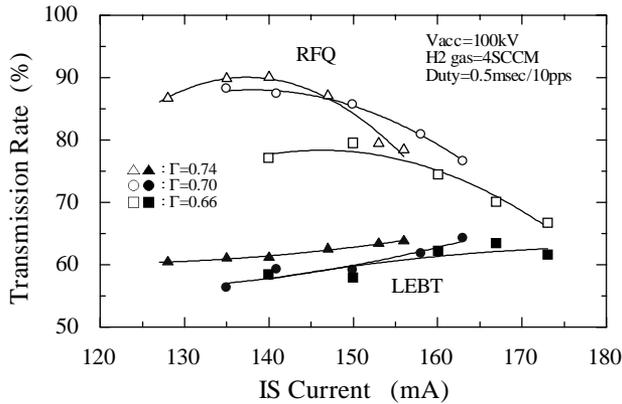
Figure 3 : Beam transmission rate in the LEBT and the RFQ as a function of the IS current.
