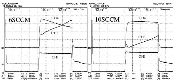
CH1 : Arc current, CH3 : Extraction current, CH4 : Negative Ion current
