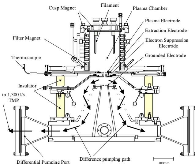
Figure 7 : Schematic drawing of new negative ion source
