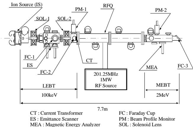
Figure 1: Layout of the 2 MeV beam line.
