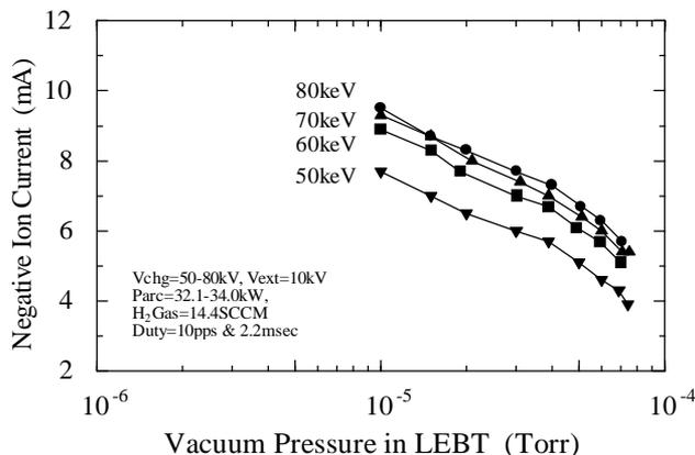
Figure 8 : Negative ion current as a function of the vacuum pressure in the LEBT
