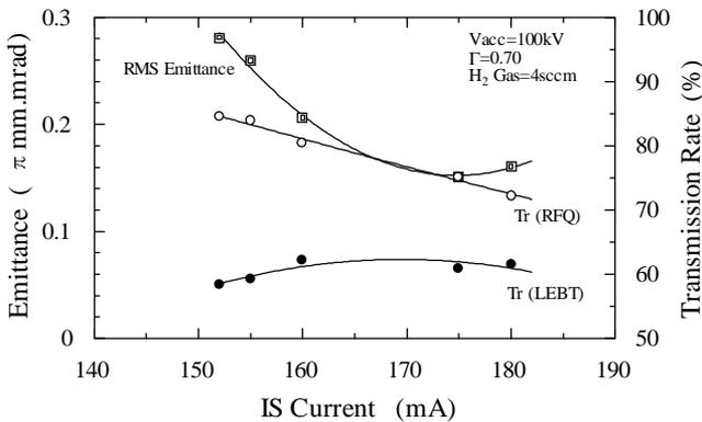
Figure 4 : Emittance of the IS and beam transmission rate in the LEBT and the RFQ as a function of the IS current.
