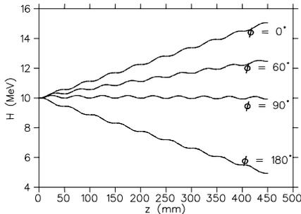
Figure 1: Energy gain of electrons in the RTM cavity. Injection at different phases  $\phi$ , at 10 MeV. Curves presenting Hamiltonian, GPT and Parmela calculations are hardly distinguishable.
