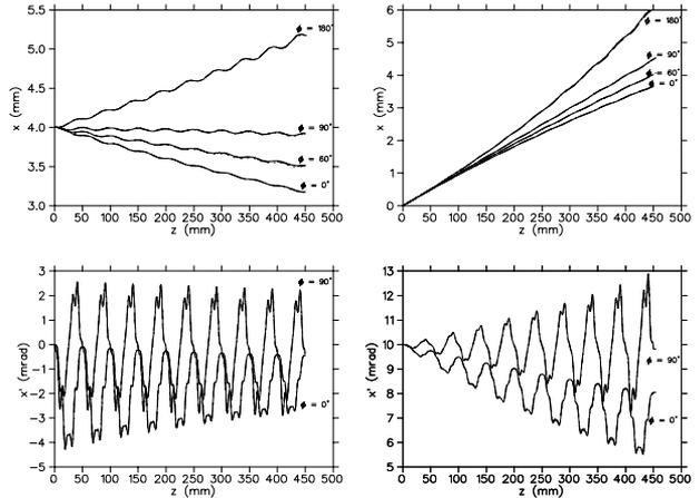
Figure 2: Electron trajectories in the RTM cavity. Injections at different phases (indicated in the figure by  $\phi$ ), at 10 MeV. Hamiltonian, GPT and Parmela calculations are hardly distinguishable.
