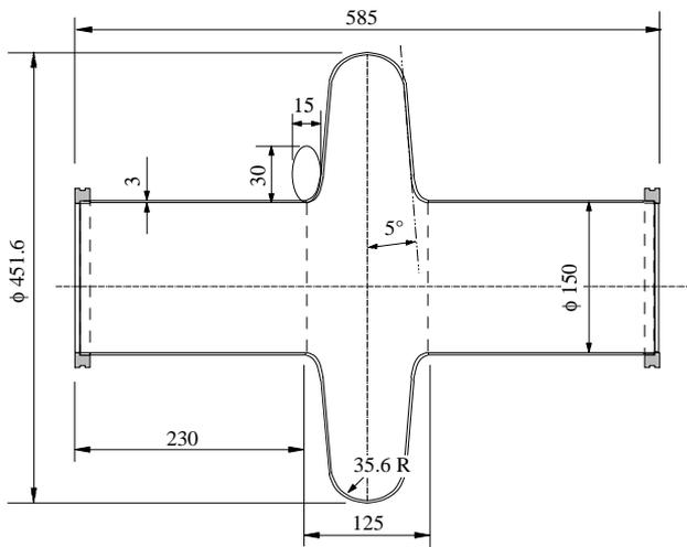
Fig. 1 Designed shape of 600MHz  $\beta=0.5$  bulk Nb single-cell cavity. (Proton energy range: 145 MeV)
