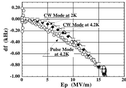
Fig. 5 Resonant frequency variance as a function of the peak surface electric field (Ep)
