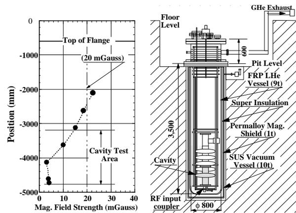
Fig. 2 Cross-sectional view of the cryostat and residual magnetic field strength in the cryostat
