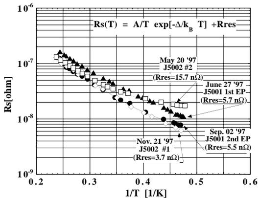
Fig. 4 Temperature dependence of surface resistance at J5001, J5002 Cavities
