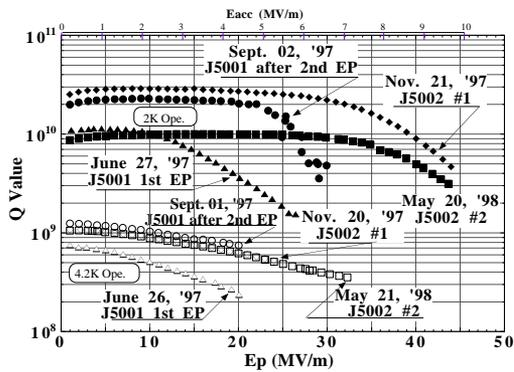
Fig. 3 Q values of the J5001, J5002 cavities as a function of peak surface electric field (Ep)
