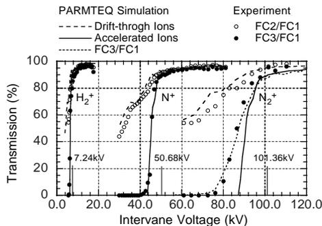
Figure 2: Transmission of the RFQ vs intervane voltage.
