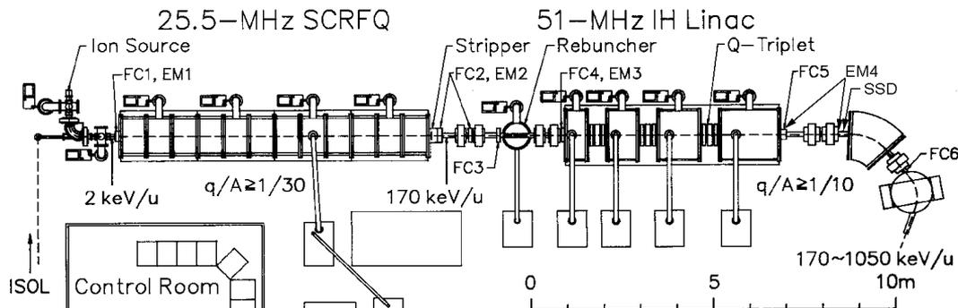
Figure 1: Layout of the RNB linac system.
