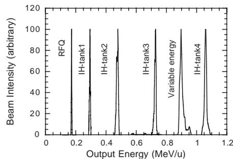
Figure 4: Energy spectra for six operating modes.
