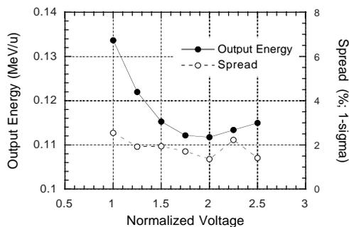
Figure 6: Energy and its spread vs normalized voltage.
