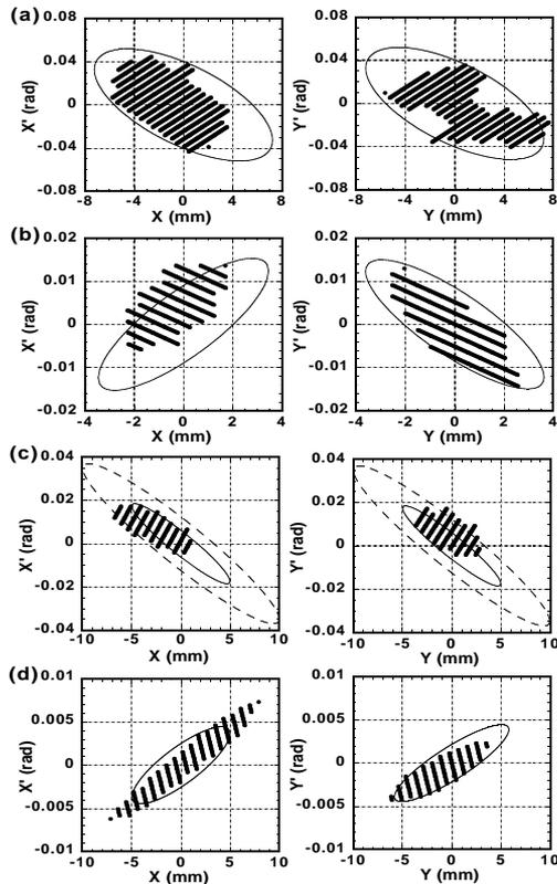
Figure 5: Emittance profiles at (a) RFQ entrance, (b) RFQ exit, (c) IH entrance and (d) IH exit.
