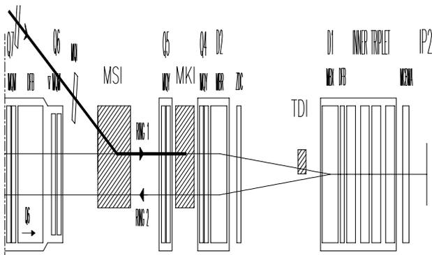
Figure 3: Schematic horizontal view of LHC injection (TI 2)
