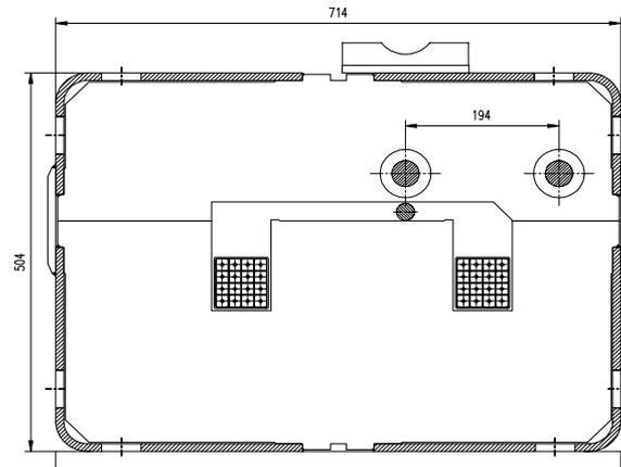
Figure 4: Cross section of steel septum magnet
