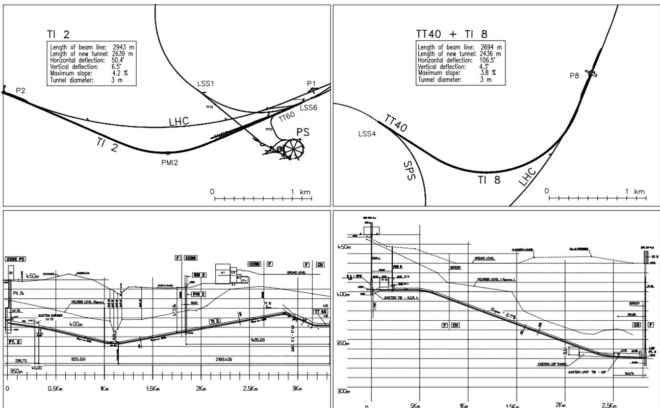
Figure 1: Geometrical layouts with main parameters (top) and vertical profiles (bottom) (TI 2 left, TI 8 right)
