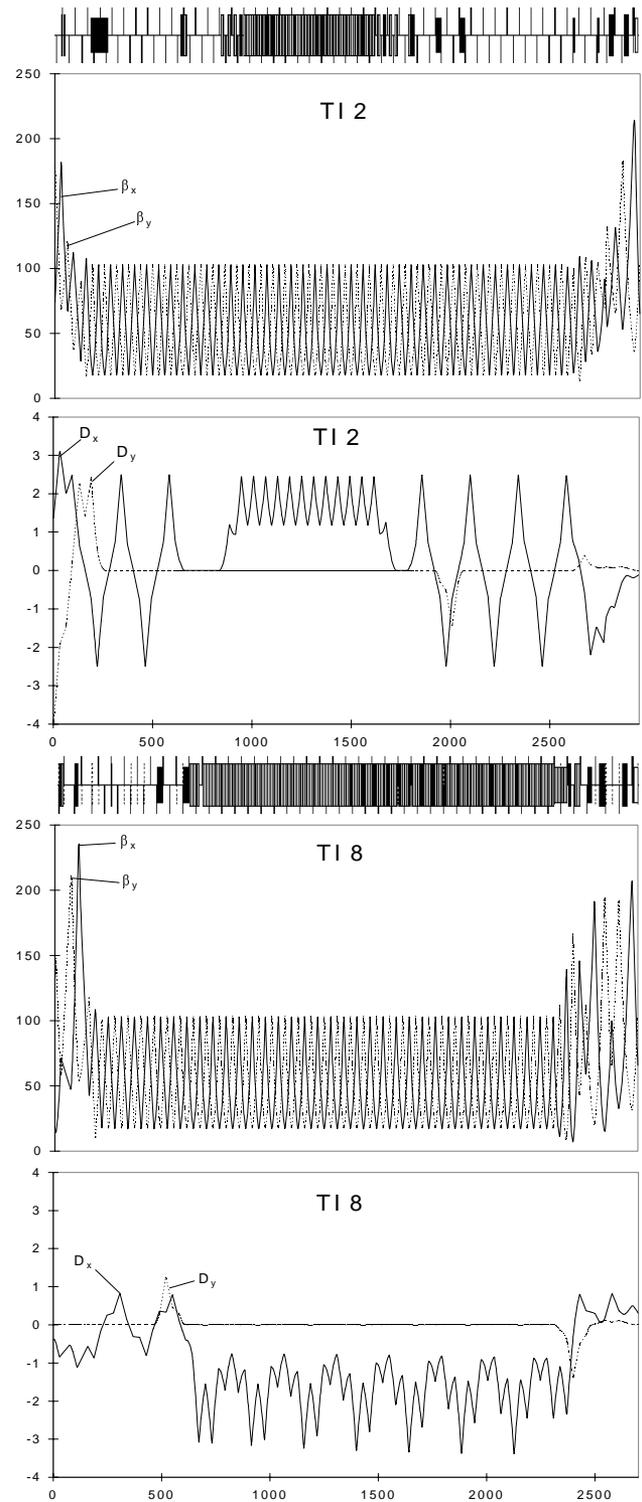
**Figure 2: Sequence of elements, betatron and dispersion functions (all values in m) for TI 2 and TI 8**
