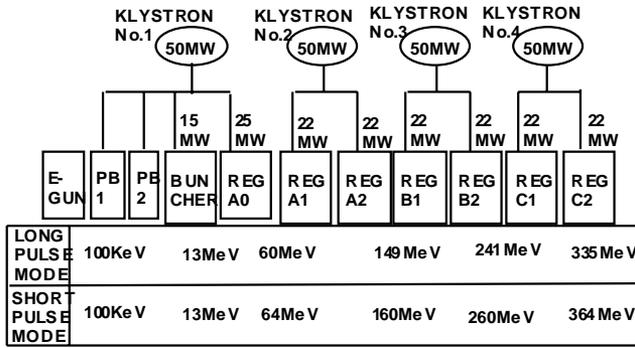
Figure 2 Energy Gain Diagram
