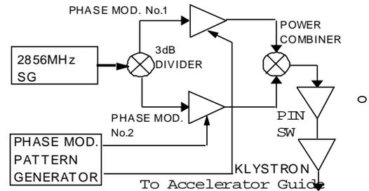
Figure 6 Energy transient Suppression by RF amplitude modulation
