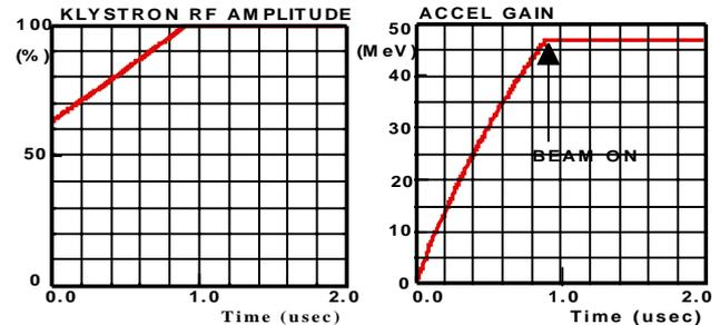
Figure 7 Energy transient Suppression by RF amplitude modulation
