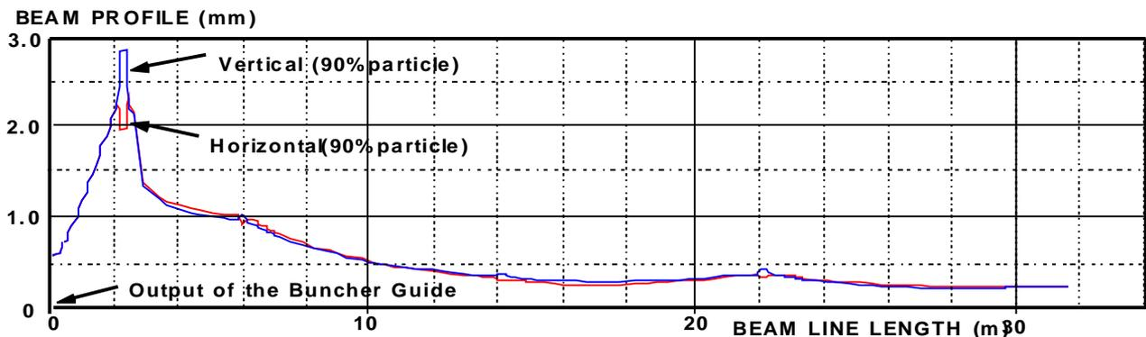
Figure 5 Beam Transport Simulation Result (Long Pulse Mode)
