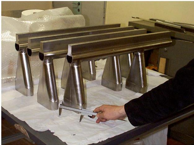
Figure 1. Bulk Nb electrodes of SRFQ2 after EB welding, ready to be modulated.
