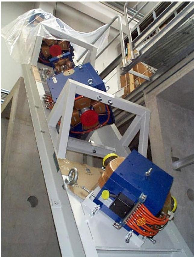
Figure 3 Achromatic U bend, aligned on a common girder, that will connect the ECR and the RFQ beam lines.
