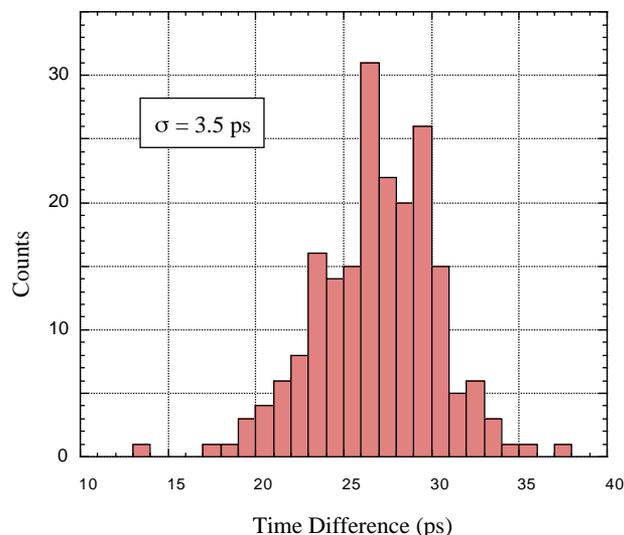
Figure:3 Histogram of time interval between laser and electron pulses.
