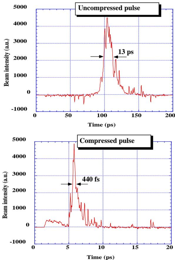
Figure:2 Measured pulse shapes with and without compression.
