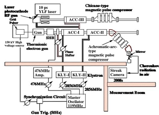
Figure:1 Upgraded second S-band linac in the twin linac system.
