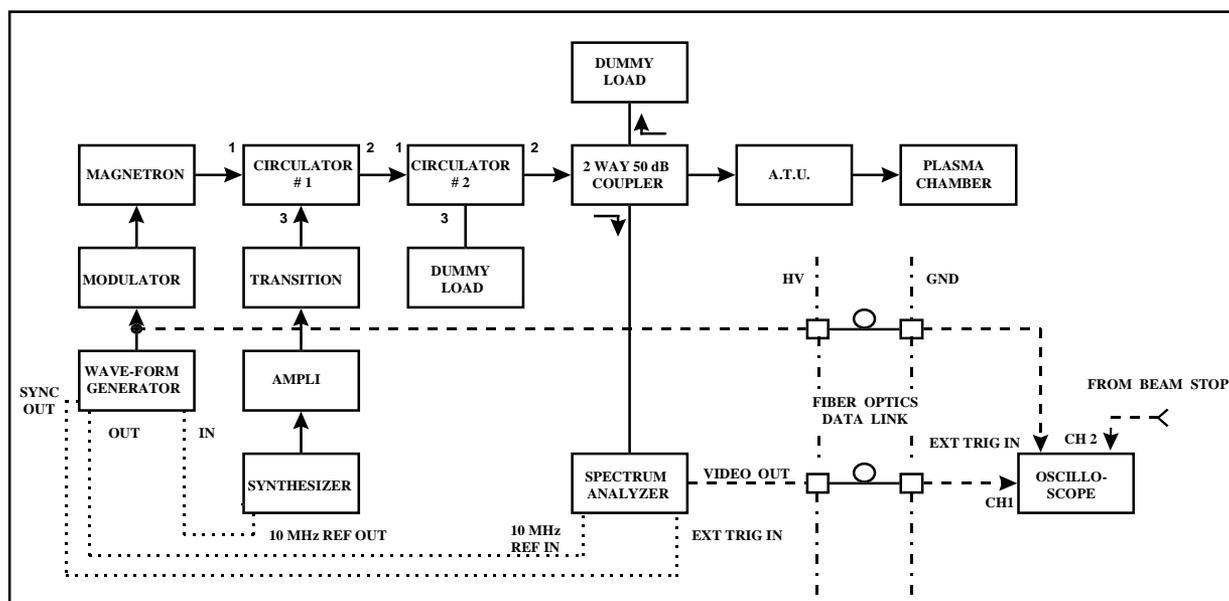
Fig. 2. RF system in pulsed mode, with injection-locking.
