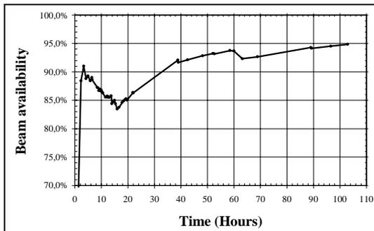
Fig.1: SILHI reliability vs elapsed run time
