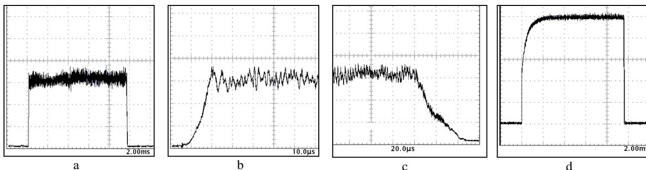
Fig. 3: (a) 10 ms plasma pulse, (b) plasma rise-time, zoomed, (c) plasma fall-time, zoomed, (d) 10 ms beam pulse
