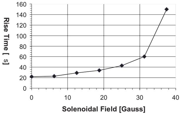
Figure 4: Measured risetime of the resistor probe signal at the onset of multipacting vs solenoid magnetic field intensity: RF frequency 480 MHz, RF forward power 50 W, 1 Hz square wave AM modulation with 10% duty cycle. The rise time measured by the oscilloscope, independent of a possible signal overshoot sometime observed, is defined as the delay required to pass from 10 to 90% of the saturation level.
