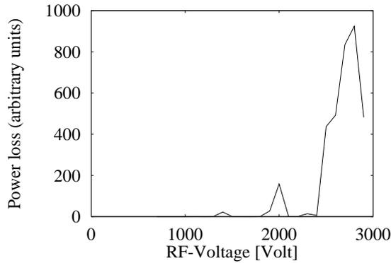
Figure 2: Simulation results for multipacting tests in a coaxial structure: power deposition (arbitrary units) versus peak RF voltage for a fixed RF frequency of 500 MHz.
