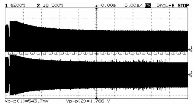
Figure 5: Multipacting tests in a warm dipole magnet: deposited power (top, 2.5 W peak) and transmitted signal (bottom) measured during a 50 s ramp of the dipole field from 100 up to 7800 Gauss. The dip on the left corresponds to a magnetic field of 170 Gauss, when the cyclotron frequency of the electrons becomes equal to the RF frequency of 480 MHz. AM modulation frequency 20 Hz, DC-bias 100 V, RF forward power 4 W.
