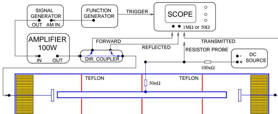
Figure 1: Experimental setup for multipacting tests.
