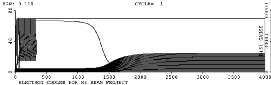
Figure 2: Electron trajectories in adiabatic expansion (unit: mm in length)
