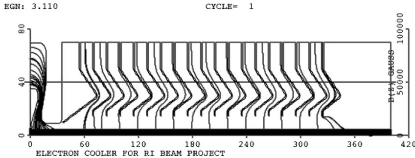
Figure 1: Electron gun with magnetic field 5T and acceleration voltage 300kV (unit: mm in length)
